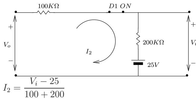
$$V_o = 25 + I_2 \cdot 200 = 2I + I_2 \left( \frac{V_i - 2I}{30I} \right) \Rightarrow V_o = \frac{2}{3}V_i + \frac{2I}{3}$$
