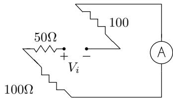
$$I_{l \ max} = \frac{V_{i \ max}}{100 + 100 + 50} = \frac{V_{i \ max}}{250} = \frac{100}{250} = 0,4A$$
